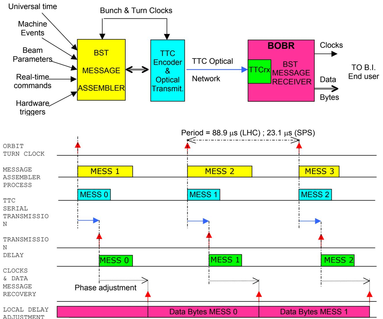
Figure 4 : Basic architecture and transmission sequence of BST Messages
