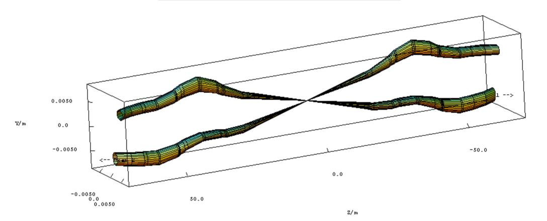
Beam separation and 3D envelopes  $(1 \sigma)$  around IP1 for LHC version 6.4 collision optics (courtesy John Jowett).
