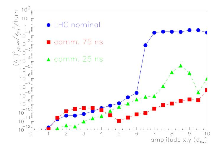
LHC diffusive aperture from parasitic beam-beam encounters for 25 ns bunch spacing with new nominal crossing angle and nominal intensity (solid blue), commissioning intensity (dashed green) and 75 ns spacing with reduced crossing angle of  $250 \,\mu$ rad (dashed red) (F. Zimmermann).
